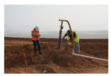
CARB inspectors detecting methane at a landfill gas collection well
