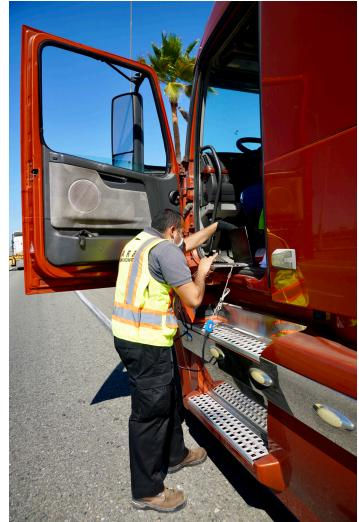
CARB Enforcement staff reading OBD data during a roadside inspection
