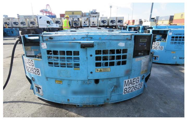
A line of TRU generator sets during an inspection at the ports
